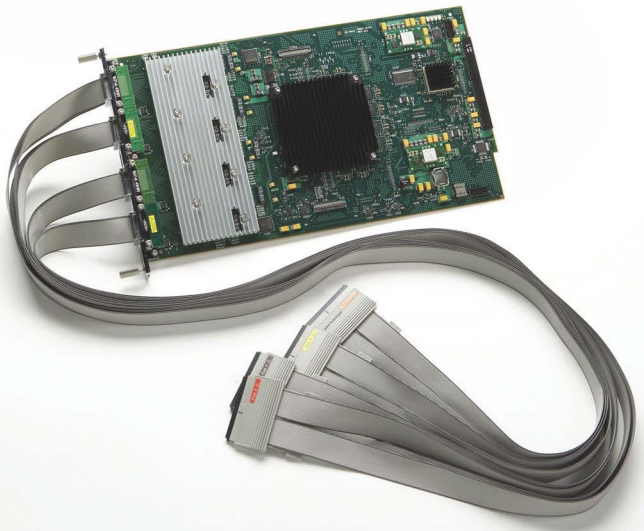
The 68-channel 16962A module, which plugs into the manufacturer's logic-analyzer mainframes, triggers on and captures DDR3 bus transactions at 2G transfers/sec in the state-analysis mode.
