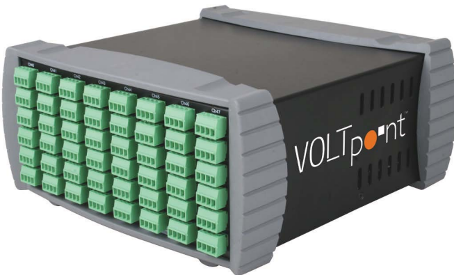
The Voltpoint series of voltage-measurement instruments for lithium-ion cell-by-cell determination offers 48 24-bit-resolution inputs over a sampling range of \pm 100V , each with its own sigma-delta ADC for direct connection to a PC through USB or Ethernet.
